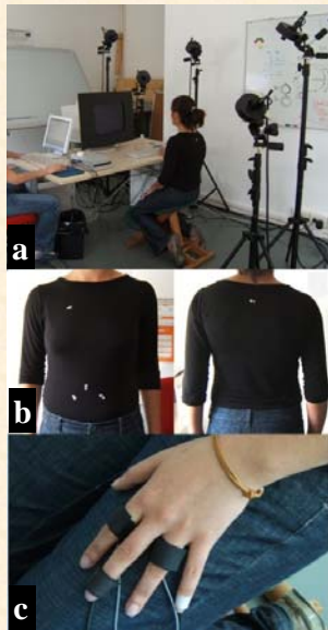
(a) View of the experimental apparatus; (b) Frontal and dorsal positions of 5 hemispheric markers whose 3D coordinates were recorded by the optoelectronic motion analyser; (c) Position of the polygraph sensors used to detect HR (middle finger), GSR (forefinger and ring-finger) and T (little finger).
